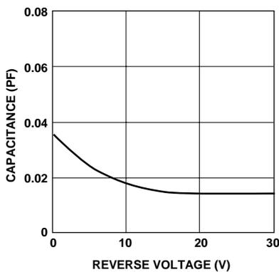
Figure 4. Typical Capacitance at 10 GHz vs. Reverse Bias.
