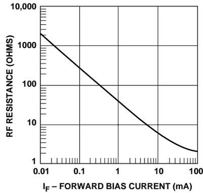
Figure 2. Typical RF Resistance vs. Forward Bias Current.
