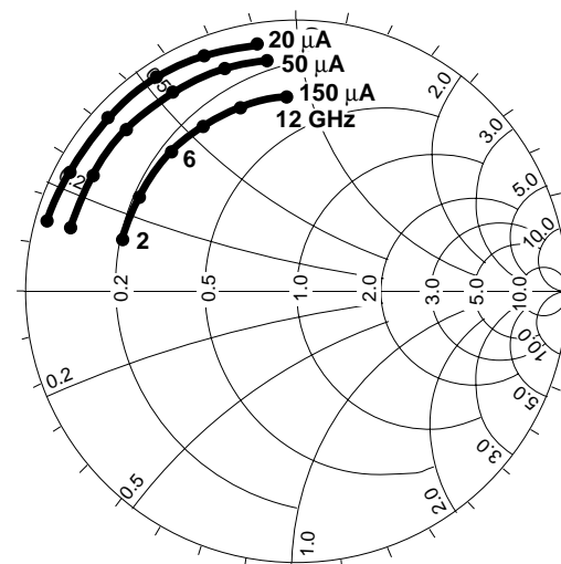
Figure 9. Typical Admittance Characteristics with External Bias. HSCH-5536.
